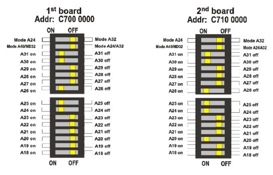
Switch Settings on Front Panel of SM128V
