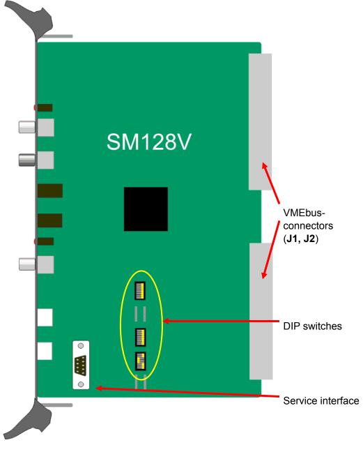
Figure 2 View on assembly side Default settings of DIP-switches: 0xE0000000
