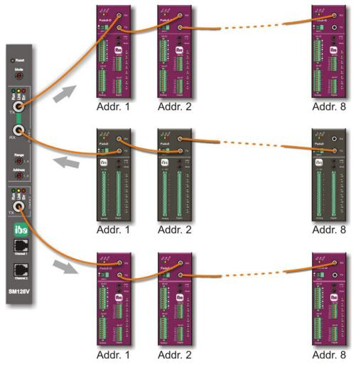
Figure 15 System topology for process i/o application with ibaPADU-8 and ibaPADU-8-O
