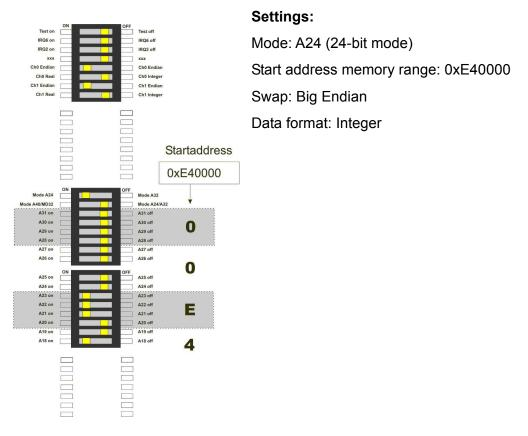
Figure 4 DIP switch, settings for ALSPA CP80/A800 (one, or first SM128V card)
