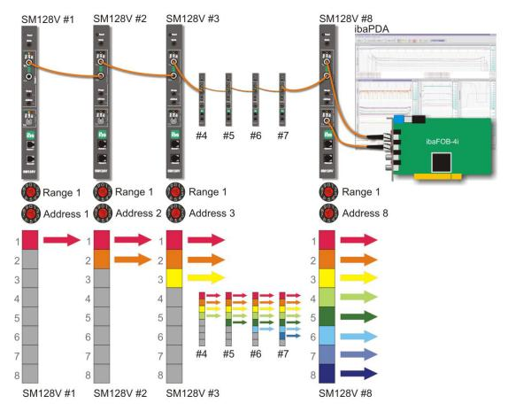
Example 1: System Topology for Daisy-Chain of 8 SM128V with Equal Ranges
